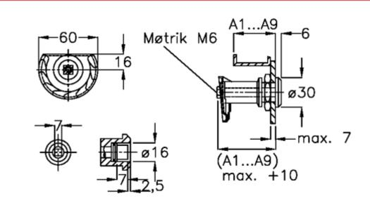
Door + frame thickness = 42-50 Measure type = A6
